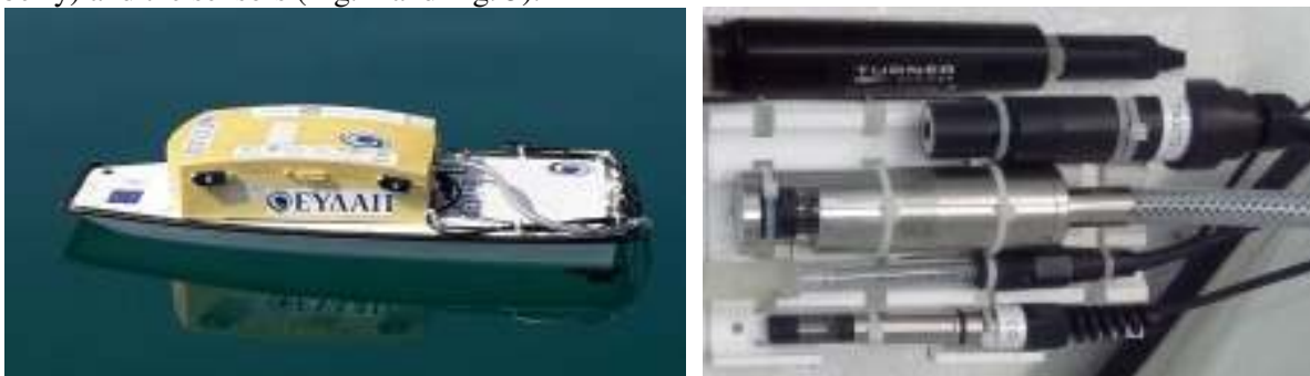
Figure 2. Autonomous Boat equipped with sensors DO, pH, ISA, EC and Chl-a (bottom to top)
