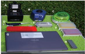
The portable lab is composed of: A) Portable PCR B) Vortex; C) Micro-centrifuge; D) Micropipette; E) Voltrax device (optional); F) Filtertips; G) Laptop; H) MinION device
