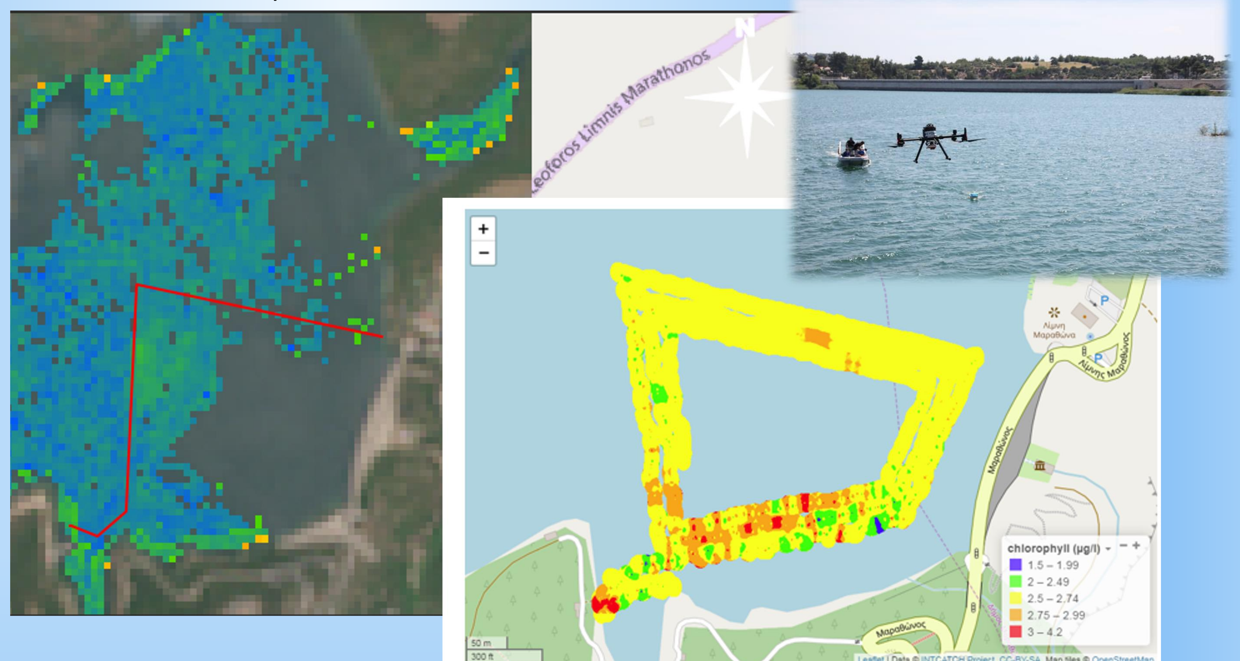
Fig.2: Mean value of chl-a along the drawn red line ( 2.66 \mu\text{g/l} ) from Sentinel-2 capture is equivalent to the yellow line ( 2.50\text{-}2.74 \mu\text{g/l} ) in capture provided by EYDAP's USV.
